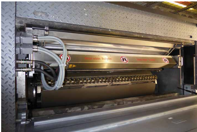
LED Powerline Focus: an UV-LED system by Eltosch Grafix GmbH
